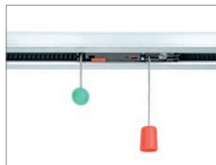
Emergency release The emergency release allows you to safely open and close your door in the event of a power cut. Pulling on the release will make the door disconnect from the opener, after which it can be manually operated.
