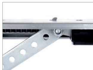
Rail with expansion kit Additional mechanical lock to protect your garage door from being opened by unauthorised persons. This locking pawl acts by engaging with the rail and by doing so preventing the door from being opened.
