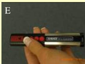
6. Take the handset. Hold the first button down. The red light in picture D starts to flash. (picture E★)
