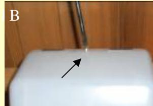
2. Remove the white cover with a small screwdriver (picture B)
