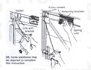
5. Pass free end of cable downward inside guide channel behind link arm. Finally, attach eye at end of the cable to hook on the roller spindle.
