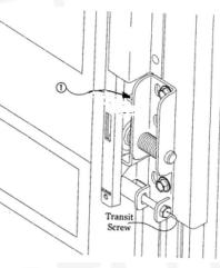
3. Undo the two grub-screws in the cable drum towards the centre of the door. The cable can now be inserted into the fixing slot. Rotate the drum so that the cable winds onto the rear of the drum. Ensure the cable runs down the inside of the track. When the cable is taut, slide the drum to the outside and tighten both grub-screws. Repeat for opposite side if required
