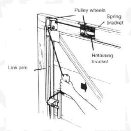
3. Loosen the side track to enable spindle to be removed. Re-position after fitting new part
