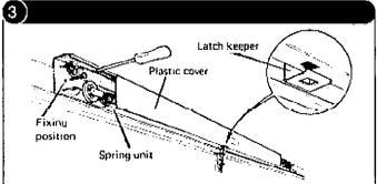
Place new spring unit onto latch keeper(s) so that the rectangular hote(s) in both spring unit and latch keeper(s) are in line. Ensure that the spring unit is parallel with the top of the door. Fix spring unit to timber head with screw provided. Repeat procedure for opposite side.
