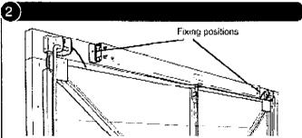
Unscrew and remove existing spring unit, also remove any pieces of cable which may still be attached to the door.
