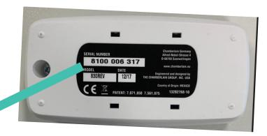
Scan or enter the serial number of the new gateway (located on the back label of the gateway).
